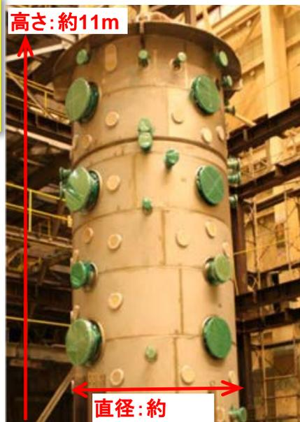
CIGMA (Containment InteGral Measurement Apparatus) の外観
